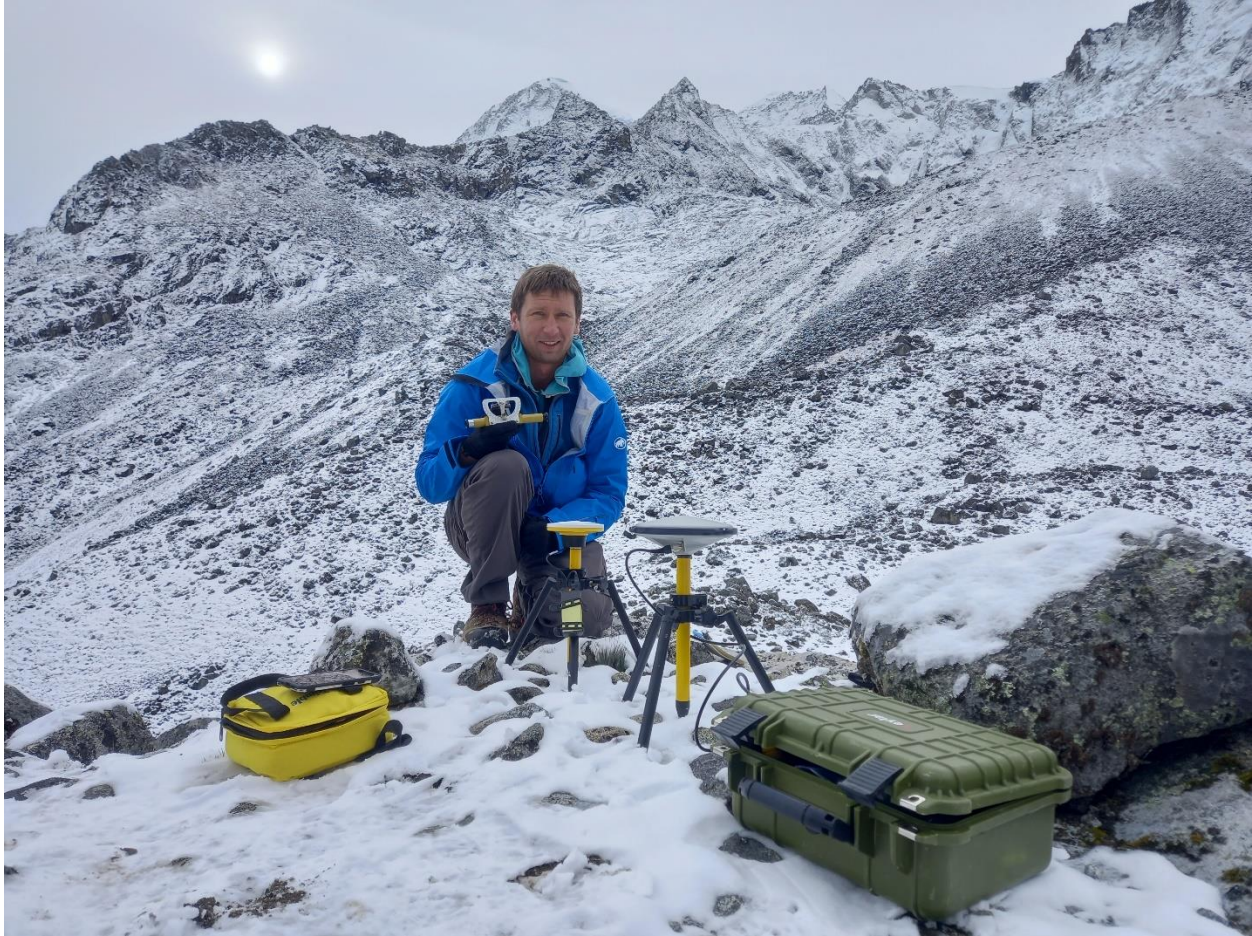
Figure 2b: The DA2 and Promark dGPS units set up at basecamp with view looking south to both summits. The Abney level is being held by the author.
