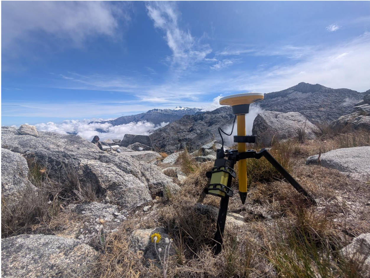
Figure 3b: The DA2 dGPS unit set up at the approach pass view Colon and Bolivar visible in the background.
