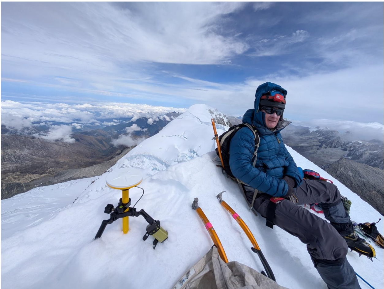
Figure 1b: The Trimble DA2 set up on the summit of Bolivar with bottom of antenna level with highest snow. View looks East with Colon visible in background.
